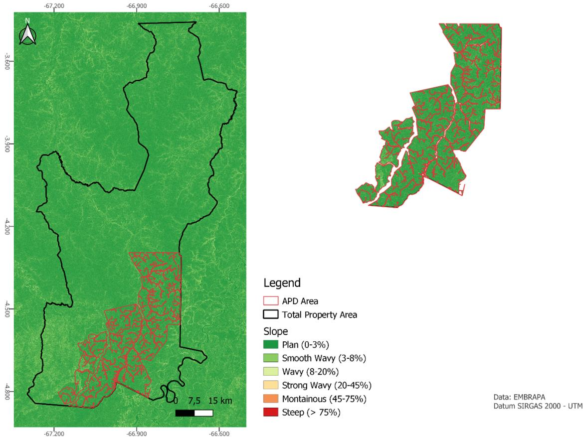
**Figure 10- Slope definition.**
